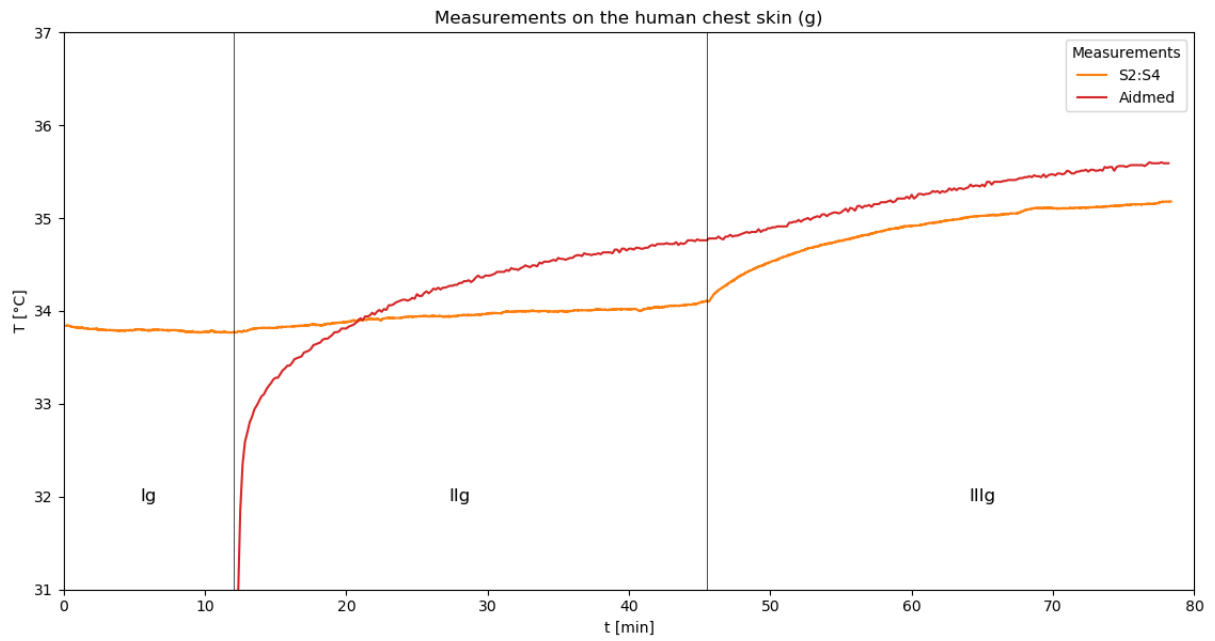
Fig. 3.15. Measurements of the human chest skin (g). Ig – only reference sensors placed on the naked chest, IIg –turned on Aidmed One placed on the naked chest, IIIg – chest covered with a T-shirt.
